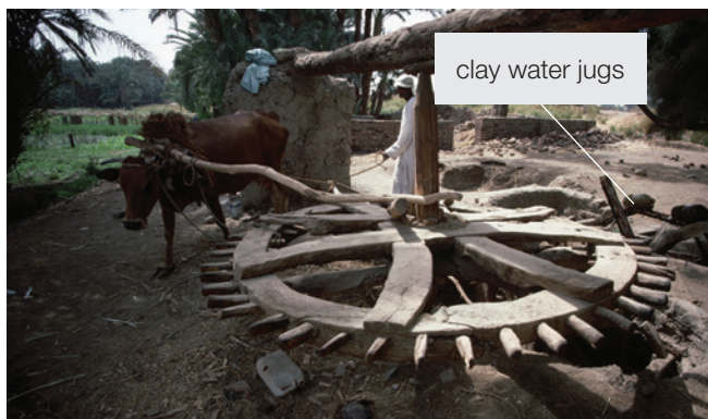
Source 14 This traditional waterwheel near Luxor, Egypt, is similar in design to those used in ancient times. The water comes out of the well on a second wheel carrying clay water jugs (shown to the right). This water then supplies the irrigation network.
